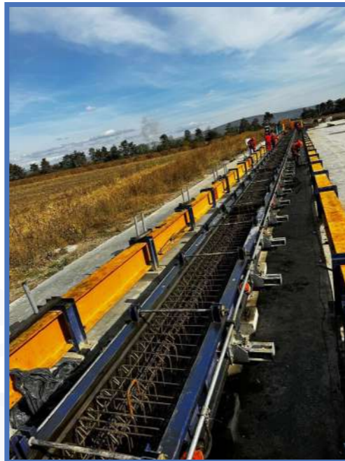
T-shaped precast concrete elements for roads and bridges (L0, L1, 2, L3) Up to 2 pieces per day.
